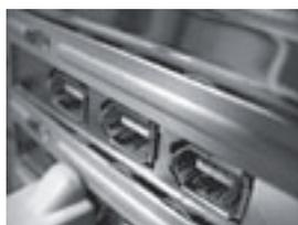
Fig 5.1 A FireWire capture card in a PC
